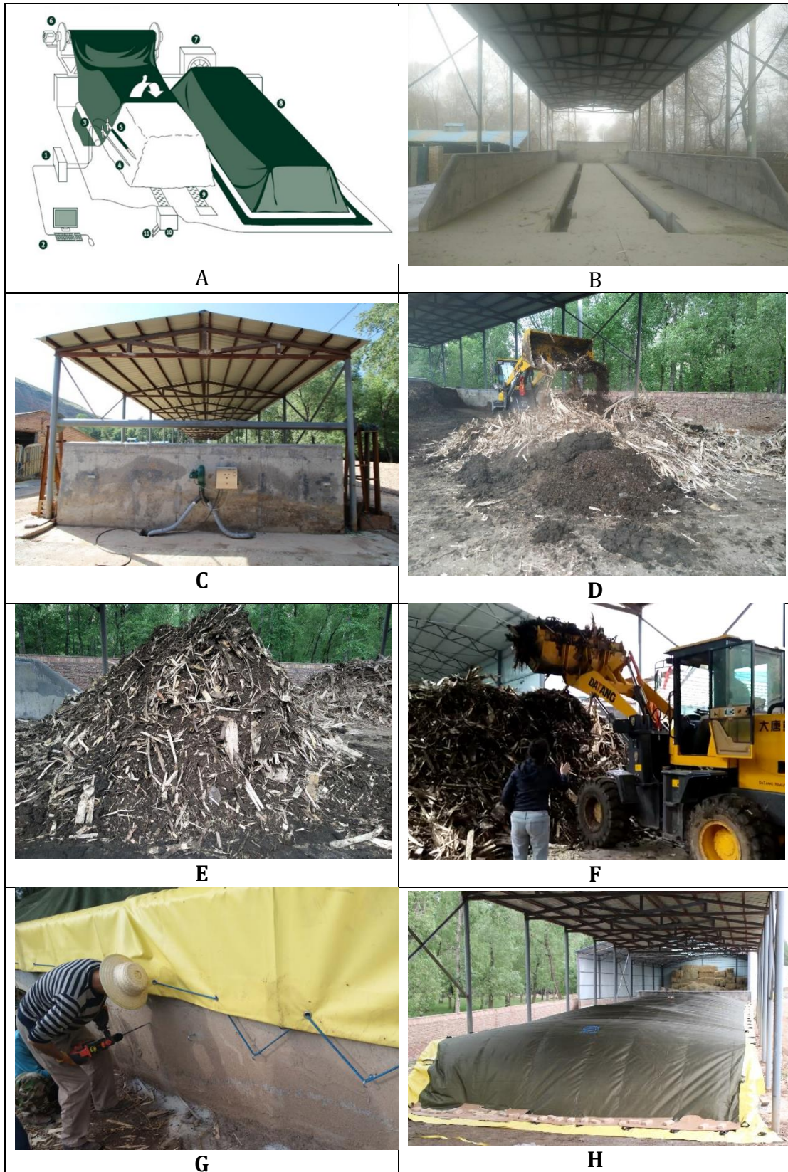
Activation process of membrane-covered compost. a) structural diagram of membrane-covered system (1. control system 2. PC 3. Rim weight 4. temperature sensor 5. oxygen sensor 6. cover handling device 7. aeration fan 8. Gore-Tex 9. aeration and leachate system 10. water trap 11. leachate collection); b) composting trough; c) fan and control system; d) mixing process with cattle manure and bulking agent; e) initial mixture; f) loading process; g) membrane sealing process; h) fermentation process
