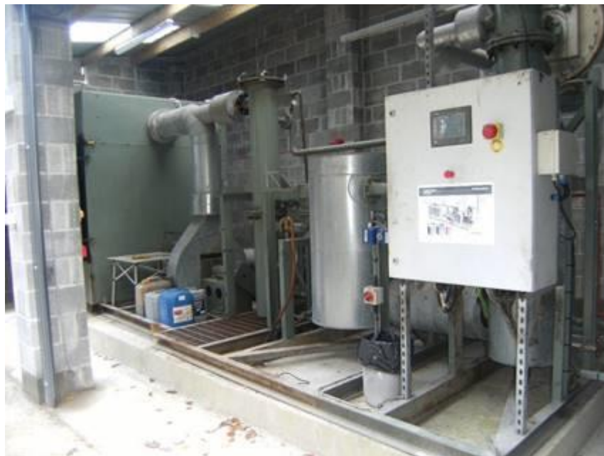
The pyrolysis unit used to produce the biochar (based at The Institute of Biological, Environmental and Rural Sciences at Aberystwyth University, Wales, UK).
